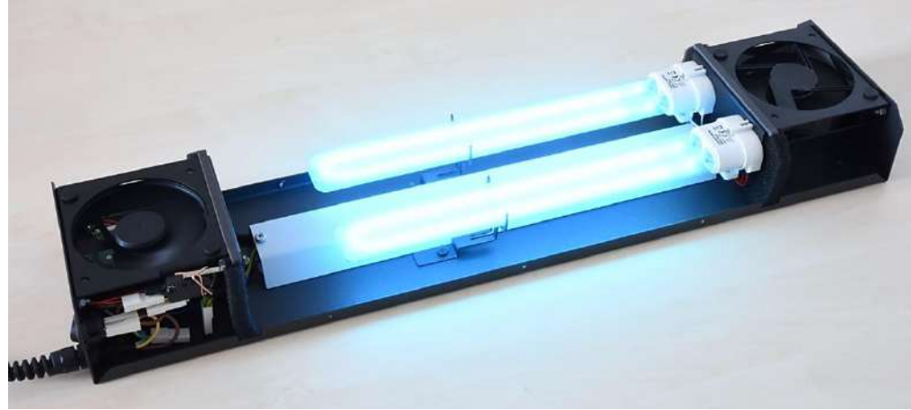
Picture above shows the UV type "C" lamps inside the LITEC SDS AIR DISINFECTION. The machine MUST NOT BE USED IN THIS CONDITION!!!
