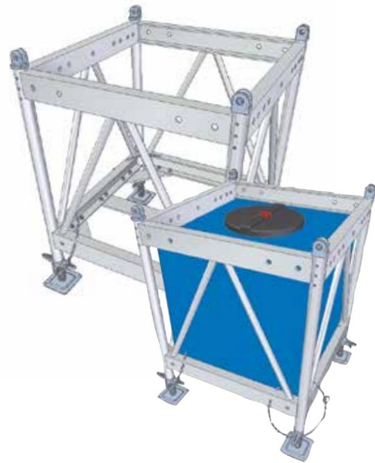
Structures are constructed out of aluminium, a light weight material which from a cost perspective remains very stable over time. The dimensions of this ballast system are 1 x 1 x 1.2 m. The tank, which can hold up to 500 litres of water, is filled at the top by hose and emptied through a bung in the bottom.
