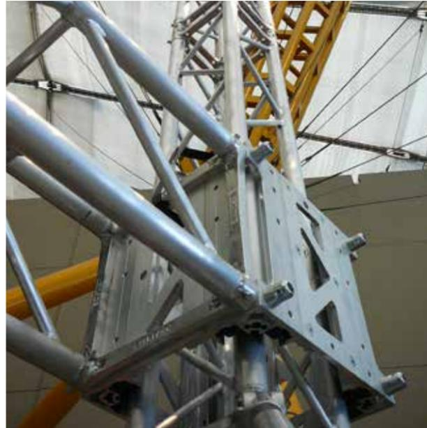
Base module for towers with frame of 29 cm sided square truss. The system comes furnished with detachable foldaway stabilizers. The multistandard sleeve block has 16 gliding wheels of high density rubber. Each foot moves both in pan and tilt so adapting to all terrain. The entire system, excluding the central truss, is formed of assembled parts, without any weldings.
