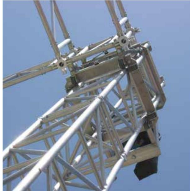
The Maxitower 52HD is a high performance, high capacity tower for your large and demanding projects. Made from EN AW 6082 T6 aluminium, it has the same dimensions as the Maxitower 52 but features  $\varnothing 60 \times 5$  mm main chords for achieving higher load capacities. Thanks to these unchanged dimensions, it's compatible with the standard Maxitower 52 sleeve block.
