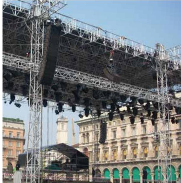
Lifter able to carry loads up to 2,000 kg. If configured appropriately, the Maxitower 40 system interfaces with all types of LITEC truss sized from 29 to 76 cm.
