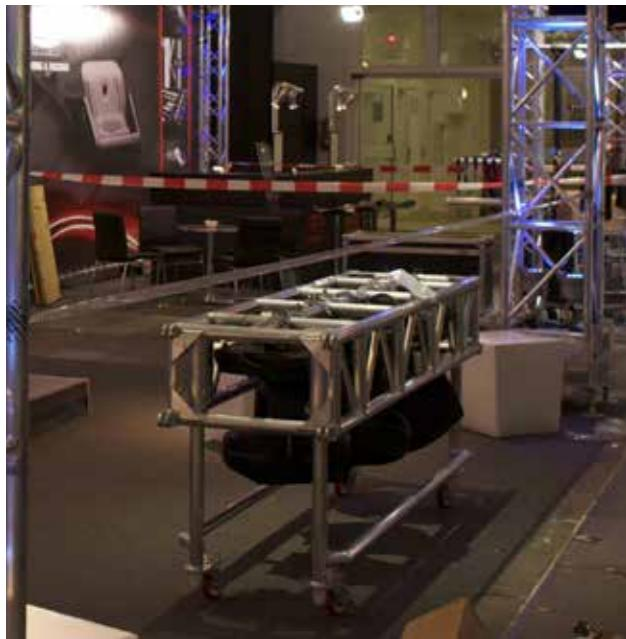
A pre-rig truss for supporting and transporting moving heads. It is equipped with 4 castor wheels for easy maneuverability and pins for the connection of truss pieces. Each truss is designed to carry a lighting bar complete with moving heads. The lighting bar is hooked onto the main chord and allows lights to move. This design reduces the amount of space required for rigging in the truck.
