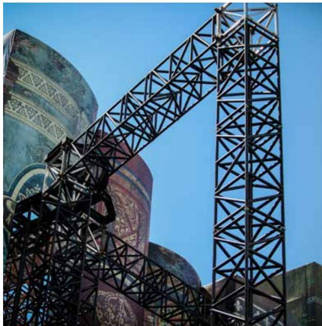
Square section High Load aluminium truss with 76 cm long sides. It is provided with steel fork connections and Ø 50 x 4 mm chords. Thanks to its elevated moment of inertia and resistance of its connections, it is mainly used in the composition of towers (Maxitower 76).
