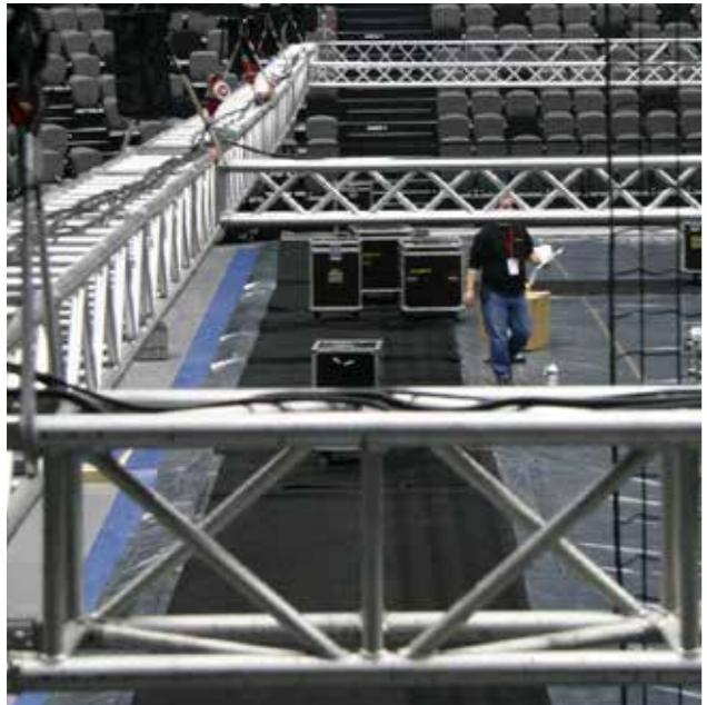
Square section High Load aluminium truss with 40 cm long sides. It is diagonalized on all faces and is provided with an aluminium fork connection. This guarantees excellent rigidity and elevated resistance in both horizontal and vertical applications despite its reduced section.
