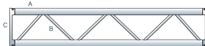
Square section aluminium truss twist-resistant version with 29 cm long sides. It substitutes the model QX30S, from which it keeps the excellent size, weight, cost and performance characteristics. It is made of 6082 alloy extruded components, with high load-bearing and twisting strength. It is a constitutive element of Unitower, Towerlift 3, and Flyintower 6-300 and Flyintower 7.5-500.
