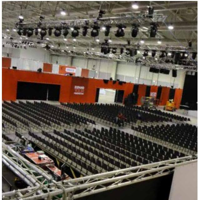
Triangular section aluminium truss with 25 cm long sides. This is the triangular version of the lightest professional structure, yet it is able to guarantee a reasonable loading capacity and span. The internal 14 mm diameter diagonal components are flush which decreases the aesthetic impact of this truss, which may therefore also be used in small areas.
