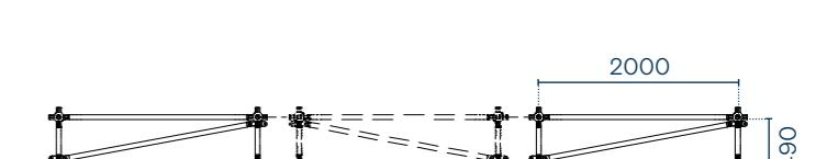
These load capacity values are only valid if the trusses are connected together every 2 metres (Lo).
