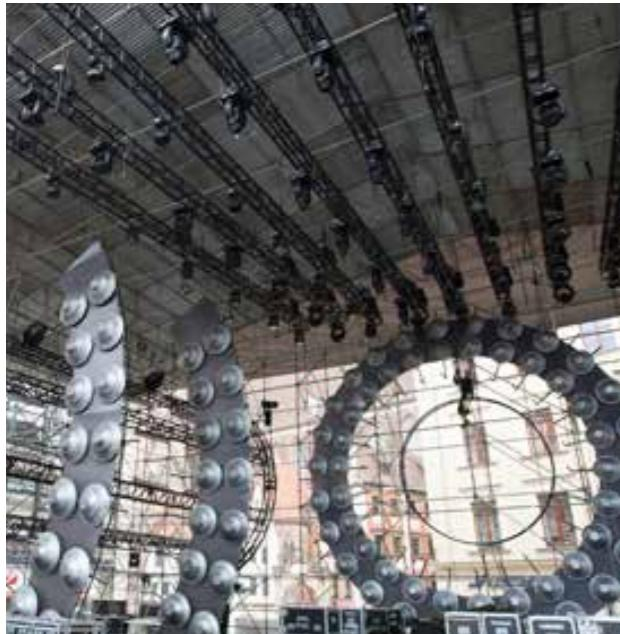
High Load 40 x 29 cm rectangular-section aluminium truss. It is the most compact truss of the High Load series with a fork connection. Suitable for quite long spans, it keeps an optimum ratio between maximum load and truss deflection. The horizontally-aligned fork ends allow the truss to be used with only minimal accessories to build grid structures.
