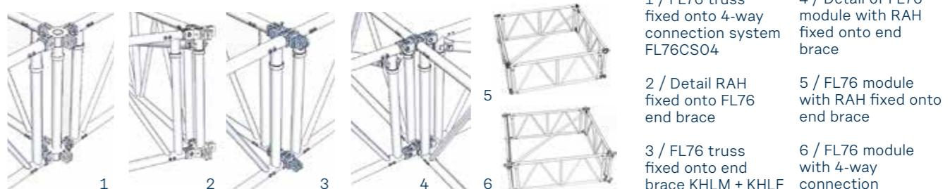
1 / FL76 truss fixed onto 4-way connection system FL76CS04
