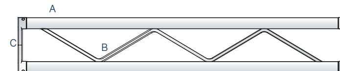
Square section aluminium truss with 25 cm long sides.
