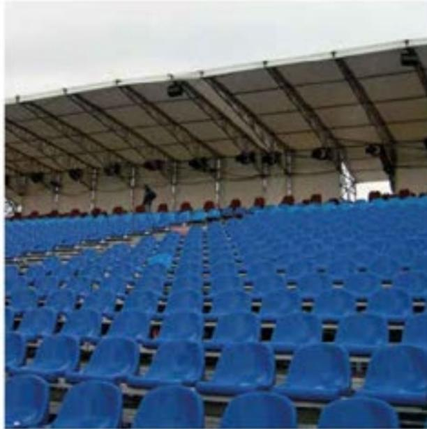
This roof system for sports derives from the LIBERA modular concept. It uses trapezoidal flat section trusses which give the structure a streamlined look and the necessary slope for water to run off. Being completely overhanging, it does not need support pillars. The maximum overhang possible is 8 metres from the back wall, provided the stand structure is sufficiently ballasted.
