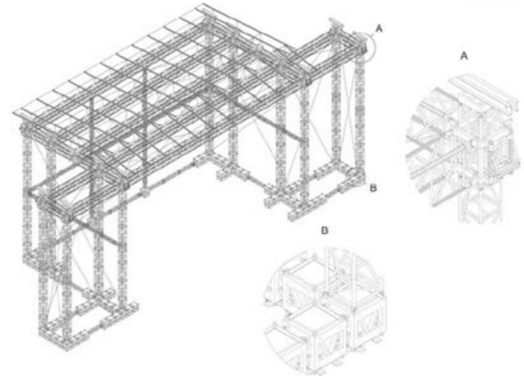
MyT Folding Steroid is a new concept in ultra high load truss that is the perfect choice for any temporary or semi-permanent structure. Made from EN AW-7003 T6 high performance aluminum alloy it maintains its form and undergoes minimal deflection even at maximum load allowing higher load capacity at longer spans than any other truss system.
