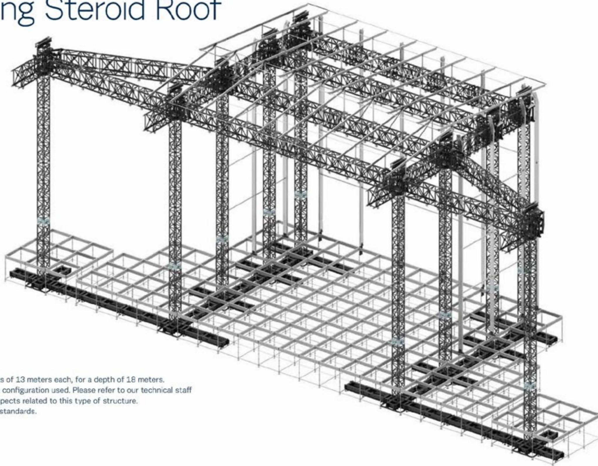
A span front of 22 meters with two side wings of 13 meters each, for a depth of 18 meters.
