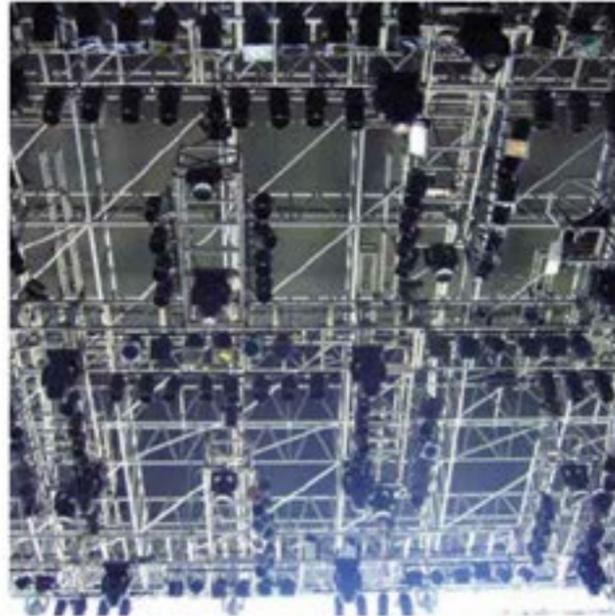
This is the largest roof system in the LIBERA range, and one of the biggest and best performing on the market. It is based on the LIBERA concept and consists of Maxitower 76 towers and LIBERA FL105 trusses. It is imposing and sturdy, and is – in itself – the most spectacular element of the show. The structure has excellent technical specifications and is highly modular.
